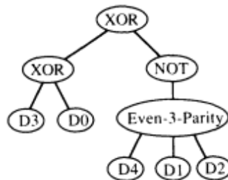
Figure 20.11 Value-returning branch of the best-of-run individual from generation 11 for the even-5-parity problem using automatic function definition.
