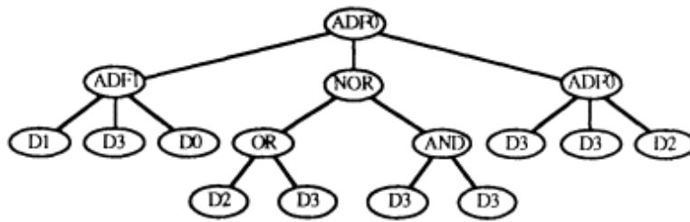
Figure 21.2 The value-returning (i.e., third) branch of the best-of-run individual uses both defined functions ADF0 and ADF1 to solve the even-4-parity problem.
